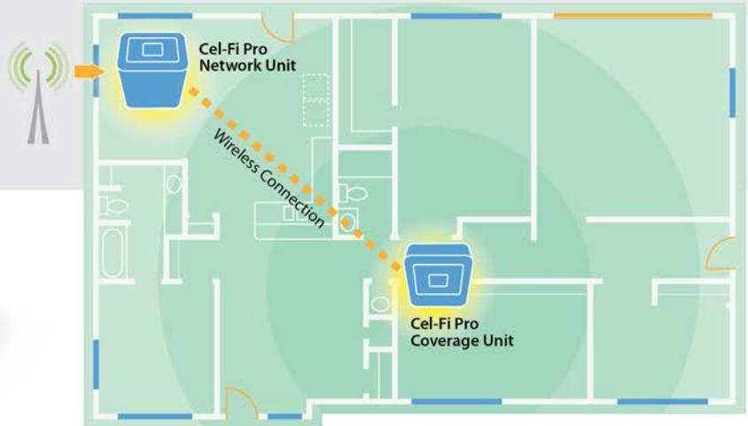
The Cel-Fi PRO is designed to dramatically improve voice and data coverage in up to four bands for 3G, 4G and LTE.
